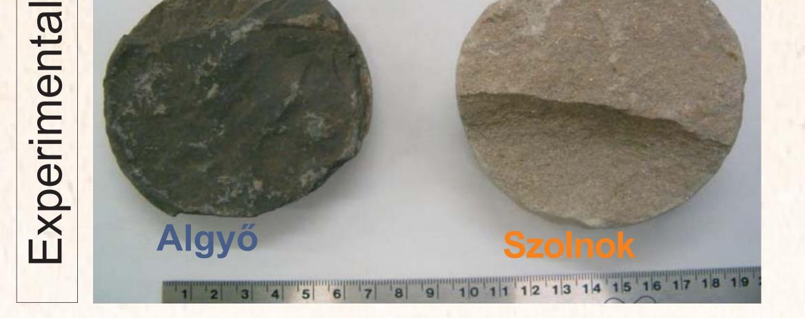
samples collected from the core shown on the Figure 3. First the rocks were saturated, in vacuum, with brine similar in composition to that observed on the field (5% NaCl eq.), then we enclosed the saturate rock sample in an INOX, pressure resistant tube and flooded the system with supercritical carbon-dioxide keeping it at 150-170 bar and 55 °C. The experiment is running while this poster is being presented. (see Figure 5)
