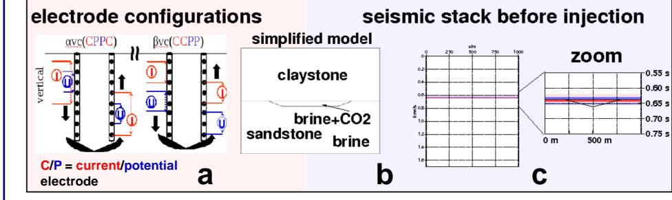
a) avcs and  $\beta$ vcs (v=vertical, c=circulating, s=symmetrical) are some of the possible applied electrode configurations.
