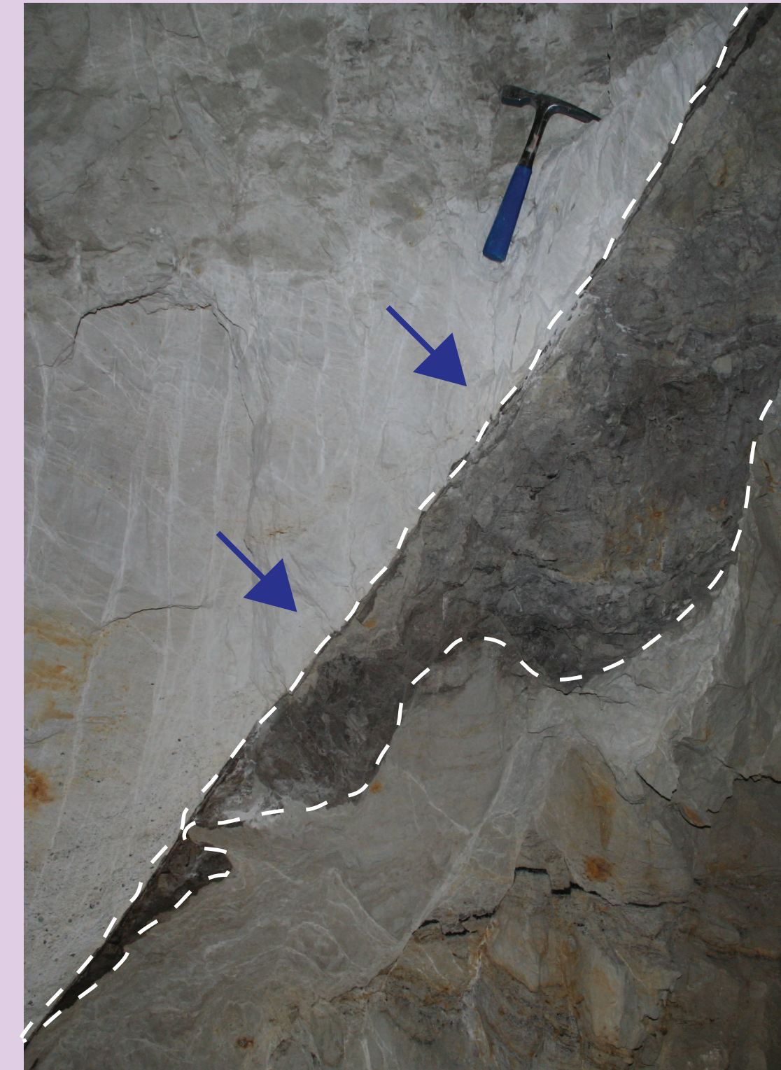
Example of clay smear, Saline Tunnel, Utah, USA
