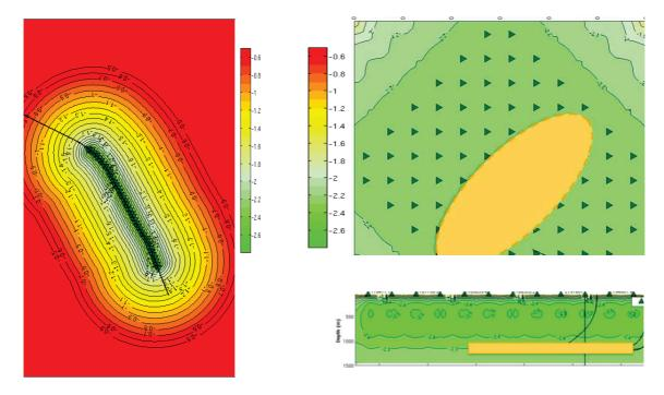
**Figure 2** Comparison of the distribution of minimum magnitude detectable with a borehole and a surface array. a) (left) horizontal cross-section through the target area including the horizontal monitoring well; low magnitude events can be detected in the vicinity of the observation well but the coverage is uneven. b) (right) same parameter mapped in a horizontal and in a vertical cross-section through the target zone: even coverage but decreased magnitude with depth.
