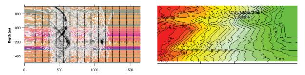
*Figure 1 a)* (*left*) waveform modelling for the analysis of waveform complexity. *b*) (right) Network sensitivity for n array deployed mid-depth above the target based on the waveform analysis.
