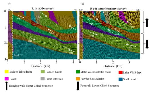
**Figure 2** The DMO-corrected stacked section along line R 141 superimposed on the geological model (courtesy of Hudbay Minerals Inc.) from a) the active 3D survey, b) the interferometry survey. The subvertical dashed line in the geological model is interpreted as a possible fault. See text for interpretation of UC, VM, and BB reflection.
