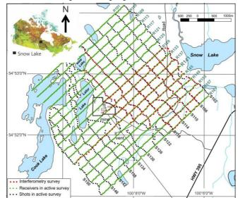
*Figure 1* Geometry of the active 3D survey and the interferometry survey in the Lalor mining area. The active and interferometry surveys cover approximately 16 km<sup>2</sup> and 4 km<sup>2</sup>, respectively. The mine area and ventilation shaft is also shown. The inset figure shows the location of Snow Lake, Manitoba.
