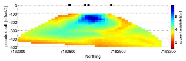
*Figure 3* Apparent resistivity section (interpolated) from measurements conducted on the Norwegian shelf, Nyegga area. Black squares mark the projection of five receivers onto the profile line.
