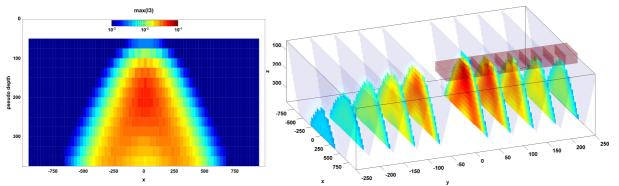
*Figure 2* Skew invariant (maximum of absolute value) for anomalous body (right, block structure), calculated for various TX-RX offsets and positions. For each TX-RX combination the according value is plotted at the midpoint between TX and RX at a pseudo depth of half the TX-RX offset (left: section at y = 25m; right: anomalous body with collection of pseudo sections).
