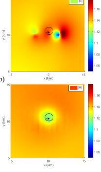
**Figure 1** (a) X-Z slice of the central part of the 3D resistivity model with the mesh used. The zoom shows a detail of the plume (yellow) in the saline aquifer reservoir (red) indicating (green triangles) two positions of a HED (inside and below the plume); (b) X-Y slice of horizontal electric and total magnetic field ratios of post- and pre-injection. The frequency is 1 Hz; the source (arrow) is located below the plume (black contour).
