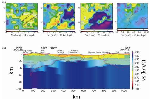
*Figure 4* Preliminar 3D shear-wave velocity model. (a) Horizontal sections at different depths. (b) Cross-section along profile shown in Figure 1a. The black line indicates the moho from Vidal et al. (1998); thered line the moho from Roca et al. (2004); and purple lines crustal bodies and moho from Carballo et al (2014).
