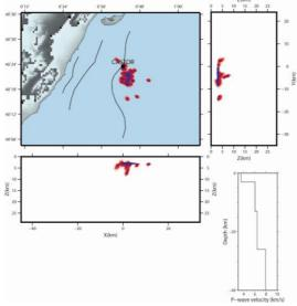
*Figure 2* Locations obtained with NonNinLoc software and the *P*-wave velocity model used (Vidal et al., 1998). Grey lines on the map are the main faults of the region.
