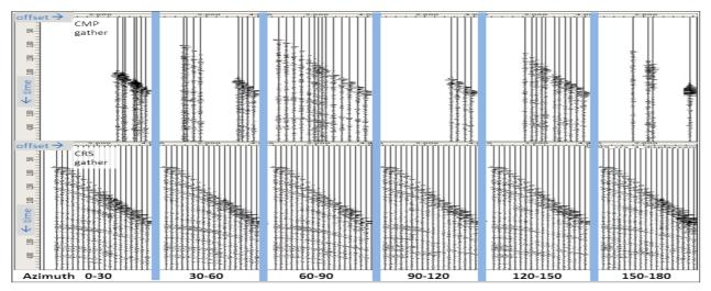
*Figure 1* Initial CMP gather (top) versus CRS gather (bottom) at the same CMP location with azimuth decomposition at intervals of 30 degrees.
