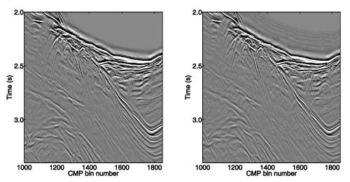
Figure 2 CRS-stack (left) and combined CRS-stack (right) from target area in Fig.1.
