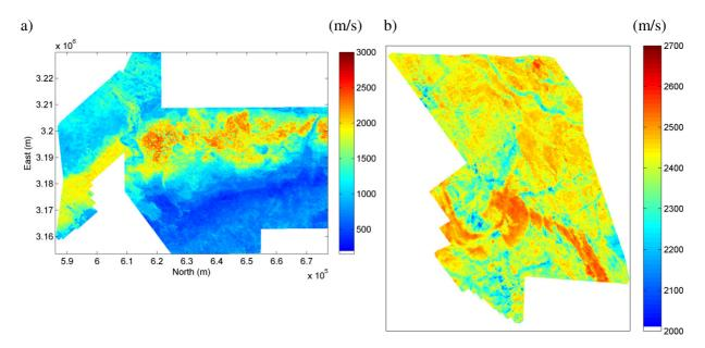
*Figure 1 a*) *S*-wave velocity at 28–35 m of depth (Boiero et al., 2013b); b) P-wave velocity at 40 m of depth below seabed.
