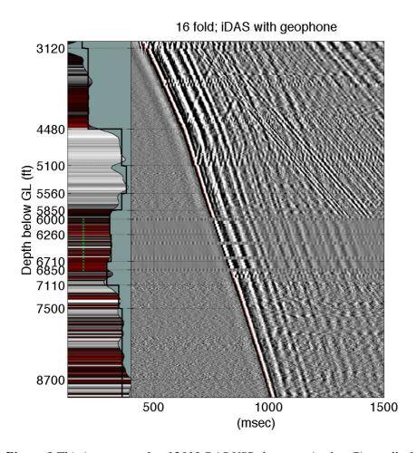
**Figure 1** This is an example of 2013 DAS VSP data acquired at Citronelle from the deepest section of the well. Data from tubing-deployed geophones between 6000-6850 ft depth is inserted (green x indicates geophone location). Shown on left side is lithology from gamma log and Vp model from DAS.
