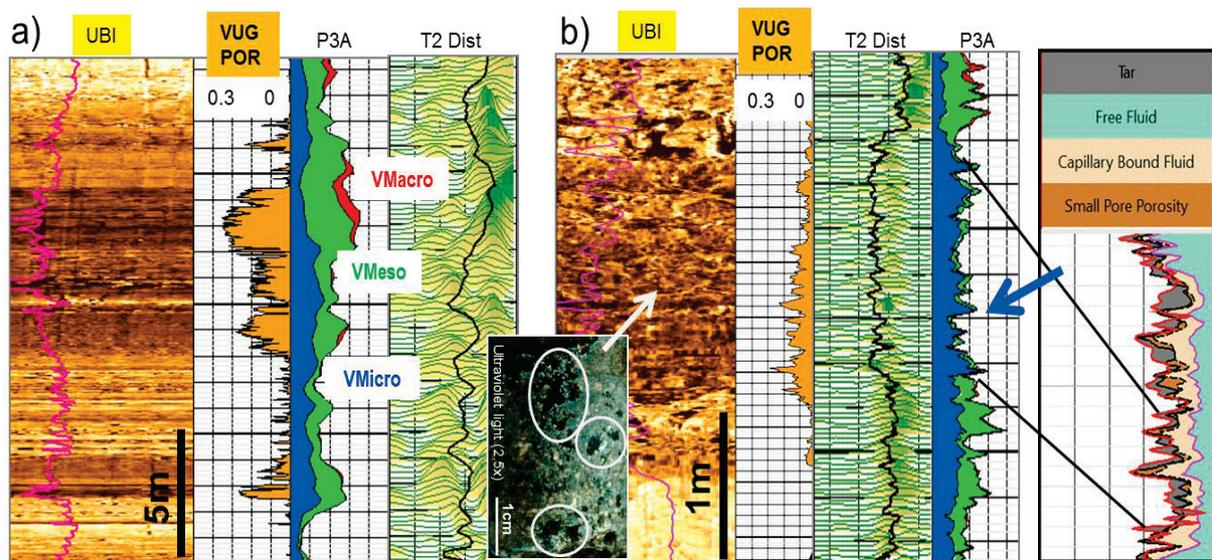
**Figure 2:** **2a)** Vuggy porosity extracted from ultrasonic image is in agreement with the NMR porosity partitioning P3A, showing high volume of macroporosity (red shading) in front of the highest density of vugs. **2b)** however some intervals show discrepancy between ultrasonic image vug porosity and NMR VMacro (blue arrow). This is due to the presence of tar or heavy oil filling the vugs (white circles on the core plug).
