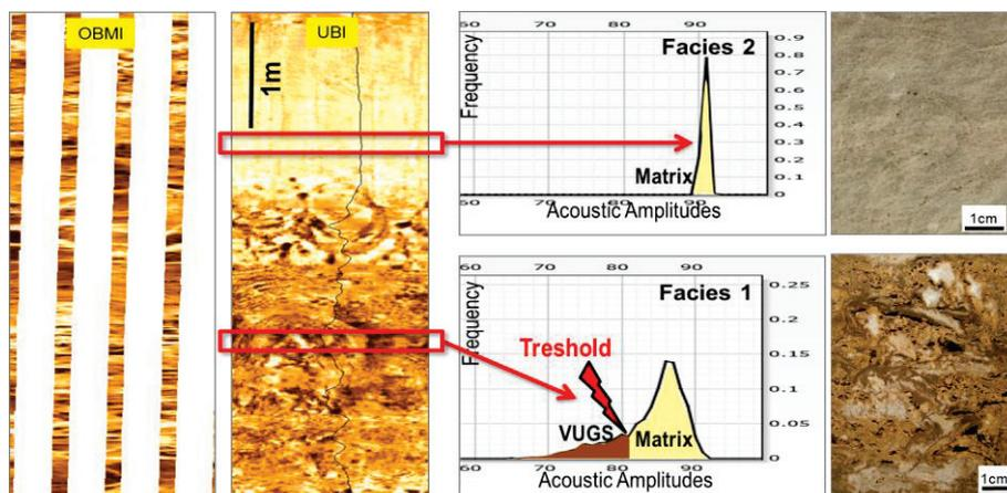
**Figure 1:** Facies 1: heterogeneous carbonate with vug porosity displaying bimodal amplitude histograms. Facies 2: homogenous carbonate with no dual porosity and unimodal amplitude histogram.
