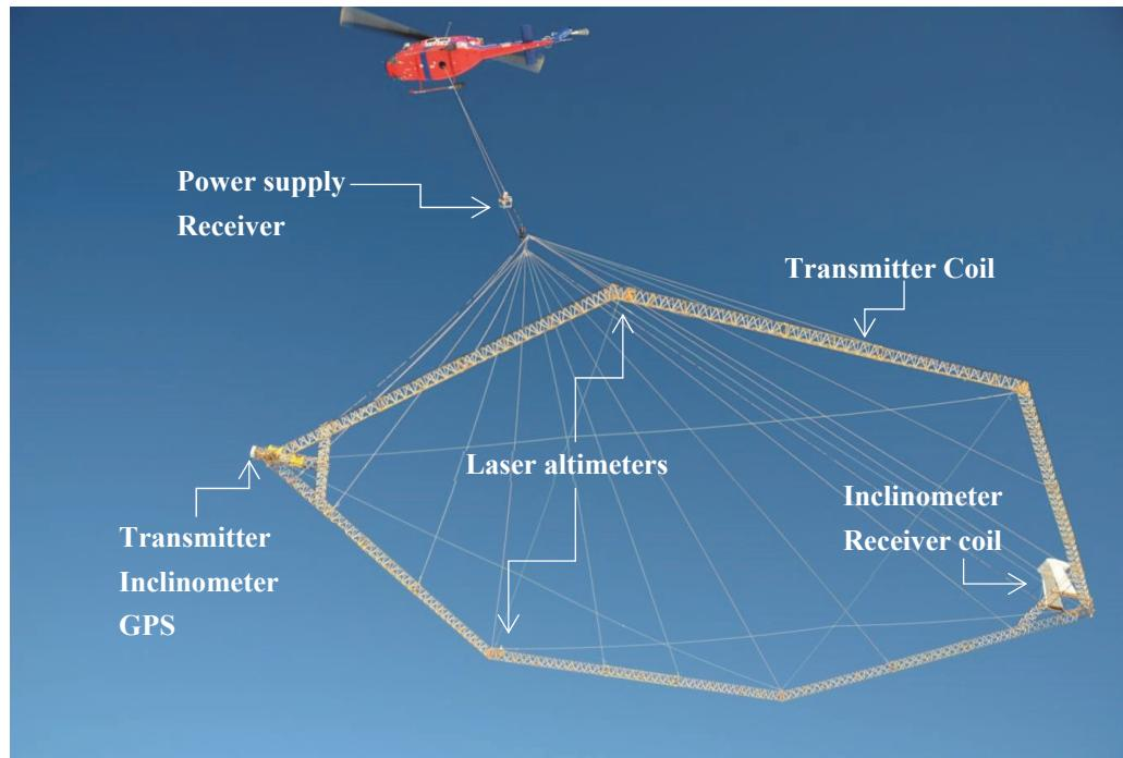
**Figure 1:** The SkyTEM system with indications of the most important devices. The frame was on the picture is outdated as the system is now operated with a composite material frame with a smaller air resistance and better stability, but the overall layout is the same.
