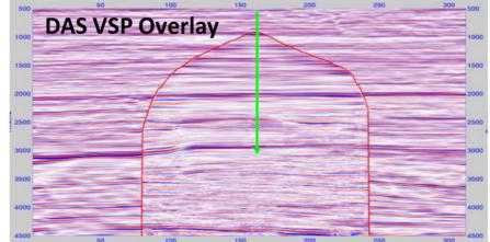
Figure 3 DAS image overlaid on surface seismic data.
