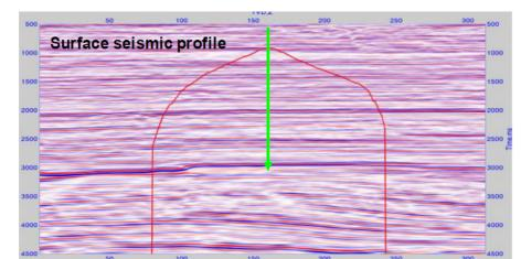
Figure 2 Surface seismic data only, red line indicates extent of DAS image.
