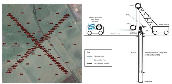
*Figure 1* (*Left*) Dynamite Shot Position Map the well is located at the centre of the 'X', (Right) Fibre Deployment Schematic.
