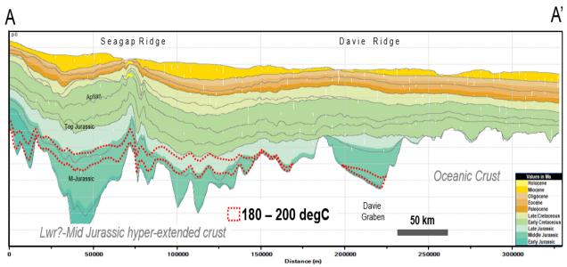
2D profile along the Tanzania margin showing the predicted position of the 200degC isotherm.
