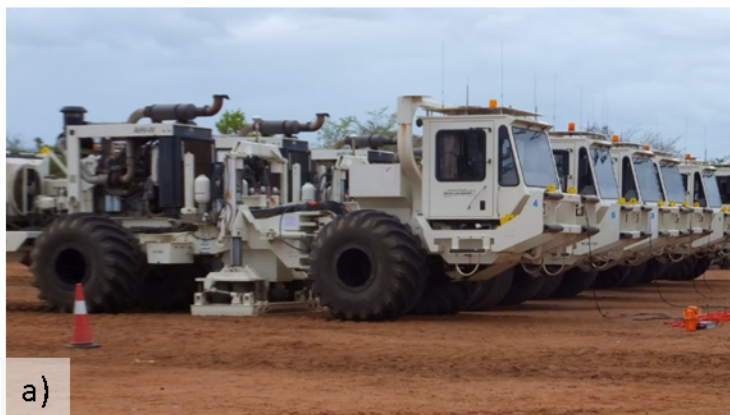
Figure 2 Source employed a) Vibroseis and Accelerated Weight Drop (AWD).
