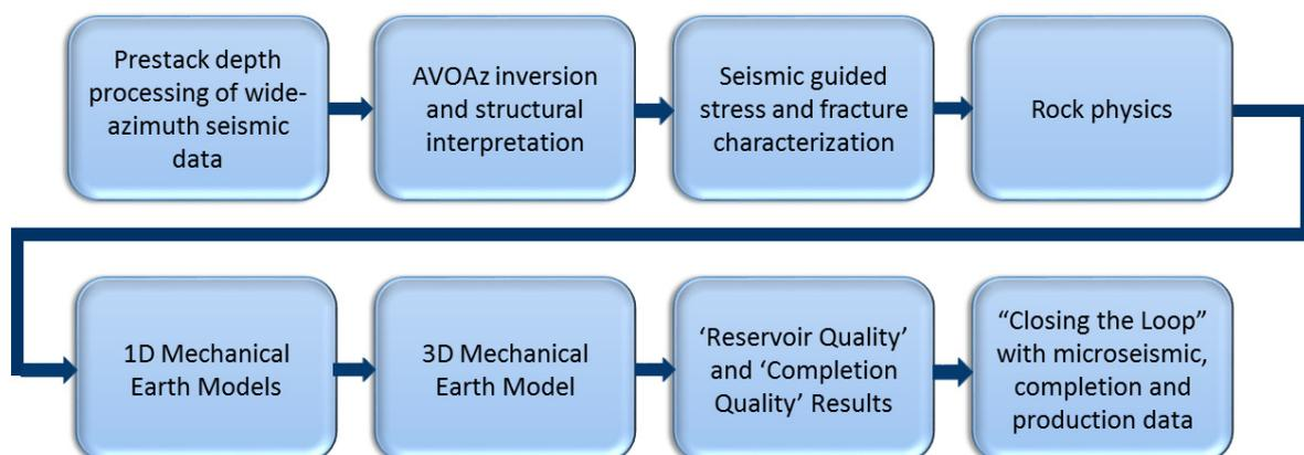
**Figure 1** Workflow used to determine in-situ stress, stress anisotropy, geomechanical properties, and the density and orientation of natural fractures in unconventional reservoirs.
