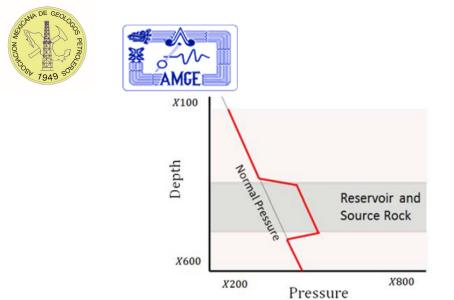
*Figure 2* Pore Pressure for Unconventional Reservoirs. (Unconventional Oil and Gas Resources Handbook-Evaluation and Development, Y. Zee Ma, Stephen A. Holditch, Elsevier, 2016.)
