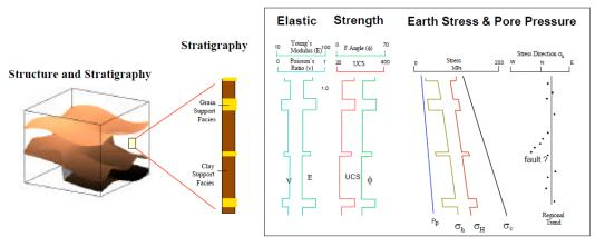
Figure 1 Mechanical Earth Model. (SPE/IADC 59128).
