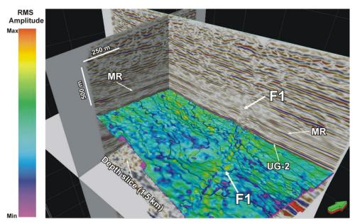
**Figure 2** 3D visualization of the 3D seismic volume showing the successful imaging of the Merensky Reef (MR), chromitite (UG-2) and its associated seismically mapped fault on the Root Meant Square (RMS) amplitude attribute display.
