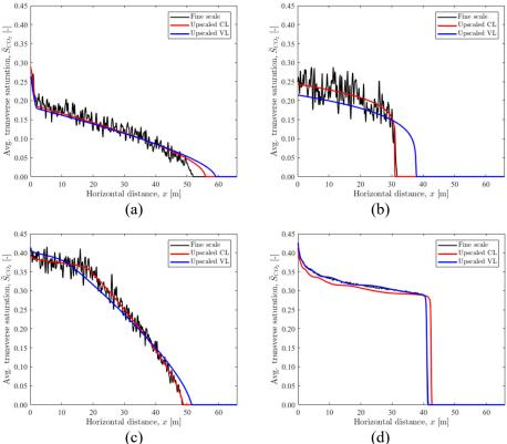
**Figure 3** Average transverse  $CO_2$  plume saturation through the domain for isotropic permeability and entry pressure fields  $r_x = r_y = 0.4m$ . (a)  $t_d = 0.1$ ,  $N_c = 0.08$ ,  $N_{gv} = 80$ . (b)  $t_d = 0.1$ ,  $N_c = 0.08$ ,  $N_{gv} = 0$ . (c)  $t_d = 0.2$ ,  $N_c = 0.2$ ,  $N_{gv} = 8$ . (d)  $t_d = 0.2$ ,  $N_c = 35$ ,  $N_{gv} = 0.05$ .
