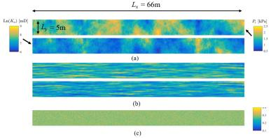
**Figure 1** (a-b) Geostatistical entry pressure fields (top) and permeability fields (bottom). (a) – Isotropic,  $r_x = r_y = 5m$ . (b) – Anisotropic,  $r_x = 0.4m$ ,  $r_y = 5m$ . (c) Porosity field.
