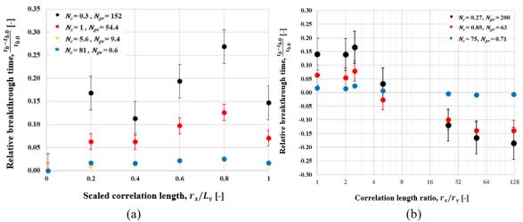
**Figure 2**  $CO_2$  plume breakthrough time as a function of correlation length,  $N_c$  and  $N_{gv}$ . (a) Isotropic correlation lengths (b) Anisotropic correlation lengths. Breakthrough times are relative to the corresponding case with homogeneous  $P_e$  field. Error bars refer to the range of breakthrough times found from 5 different geostatistical realizations (at high  $N_c$  these are within the symbols).
