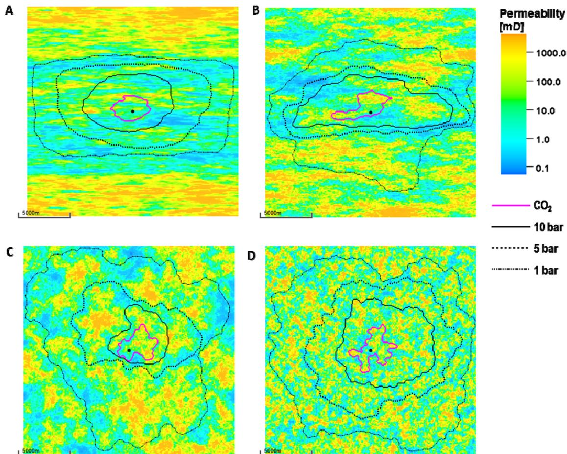
**Figure 1** Results showing the extent of the CO<sub>2</sub> saturation in all layers (pink) for four different permeability distributions (top layer only shown). Pressure increase contours displayed at 1, 5 and 10 bars.
