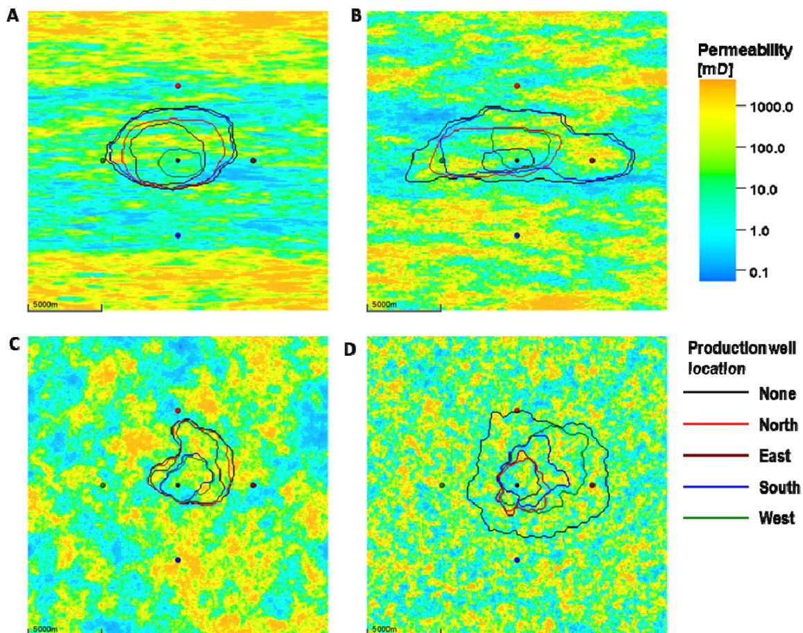
**Figure 2** Results showing the 10 bar pressure increase contour for four different production well locations. Black lines correspond to no water production, red indicates the 10 bar pressure increase contour with water production from the northern well (marked with a circle), brown from the East, blue South and green West. All production well locations are 5 km away from the injection well.
