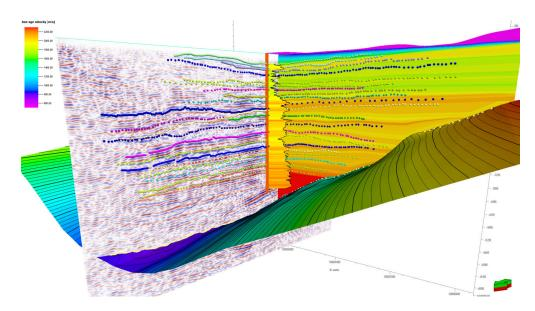
*Figure 2* Petrel snapshot of the 65 m deep geomodel. Seismic interpretation is done on the depth migrated images of reprocessed 2D seismic lines.
