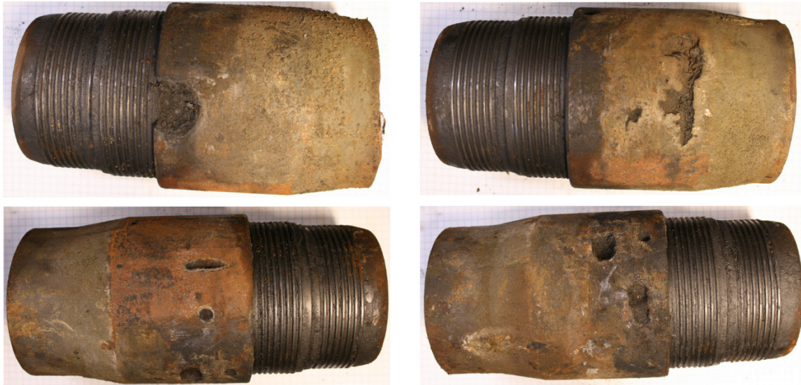
Figure 2 Photographs of 3 ½ injection tubing obtained from various wellbore depths in Ketzin well 201: (top left) from 87 meters depth; (top right) 182 meters depth; (bottom) 277 meters depth.[2]
