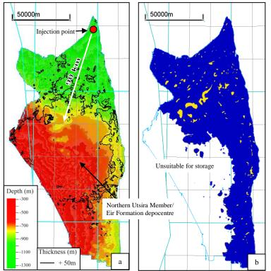
**Figure 3**  $CO_2$  storage of the Northern Utsira Member and Eir Formation. a. Depth map highlighting suitable depth areas (green) and non- suitable areas (red), with 50+ m thickness contour. b.  $CO_2$  accumulations at the top Utsira Formation.
