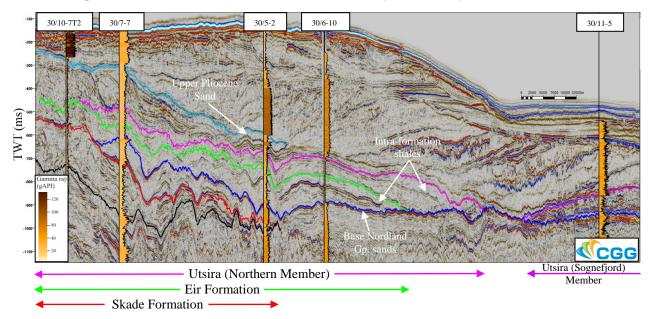
*Figure 2* Composite seismic line showing the extent and relationship of the Neogene Sands with gamma ray traces overlain. The position of the line and the formation extents are shown on figure 1.
