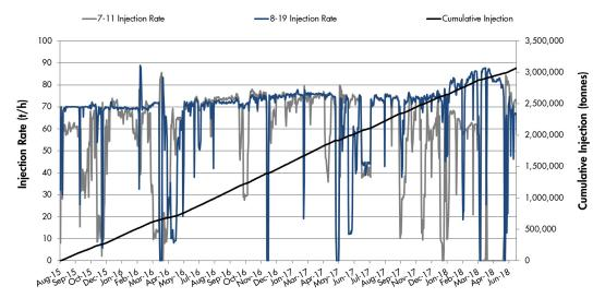
*Figure 1* Quest Injection Totals: Cumulative  $CO_2$  injected into the wells from start-up through to the middle of 2018 (right axis). The blue and grey lines show the average hourly flow rates into the two individual injection wells.
