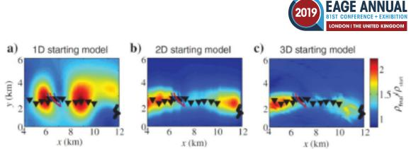
*Figure 2* Resistivity distribution inside reservoir zone obtained from different starting models, shown in terms of resistivity update done by inversion from constant resistivity at the depth level at which values are extracted (Schaller et al., 2018). Triangles indicate surface receivers. Red and blue lines indicate trajectories of a steam injection and two production wells, respectively.
