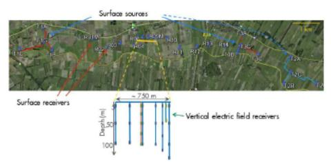
*Figure 1* Layout of trial time-lapse survey. Yellow line is Dutch-erman border. Red and blue lines indicate layout of transmitter cables.
