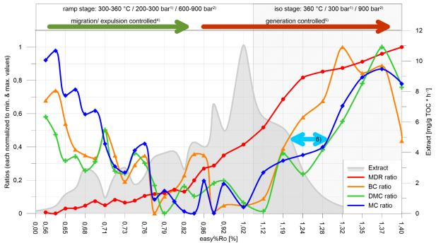
Generation & expulsion profile of an Expulsinator experiment (source rock: Posidonia Shale). Pressures (<sup>1)</sup>hydrostatic, <sup>2)</sup>lithostatic) and temperature were increased ramp-wise, followed by constant values. Symbols represent sampling points. Ratios were normalized to their respective lowest and highest values to ensure comparability.
