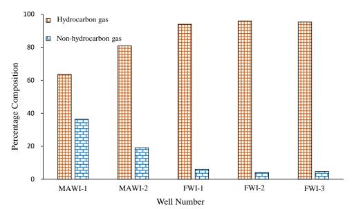
**Figure 1** Hydrocarbon and non-hydrocarbon characteristics of casing gas MAWI-1, MAWI-2: Casing gas from the well of microbial activated water injection; FWI-1, FWI-2 and FWI-3: Casing gas from the well of formation water injection; Hydrocarbon: C<sub>1</sub>-C<sub>5</sub>; Non-hydrocarbon: O<sub>2</sub> and N<sub>2</sub>
