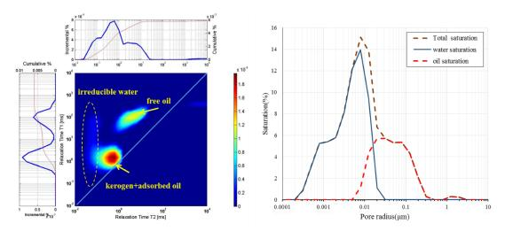
Figure 1 Representative 2D NMR image and relationships between fluid saturation and pore radius of the Qingshankou first member shale
